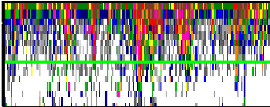
Fig. 11c. Expanded echogram showing sharp fluctuations of the bottom (indicated by the yellow jagged line representing the sounder-detected bottom). The lower solid green line is the bottom line, as detected by the software.
