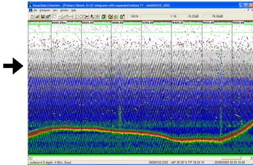
Fig. 13b. Common noise pattern as seen on a 70 kHz acoustic echogram showing noise from hydraulic winches (arrow indicating vertical spikes) during trawl deployment.
