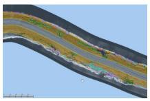
Figure 2: Example of the processed sidescan sonar imagery that has drawn polygons of different classes of substrate calculated using the SonarWiz Seabed Classification tool.
