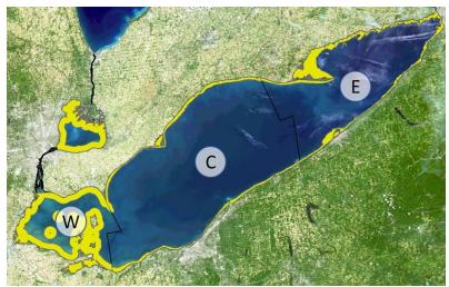
Figure 13: Lake Region and Nearshore PMA Layers. Lake regions layer delineates West(W), central (C) and East (E) basins, Nearshore defined using a 5km buffer in West Basin and the 10m depth contour in central and east basins
