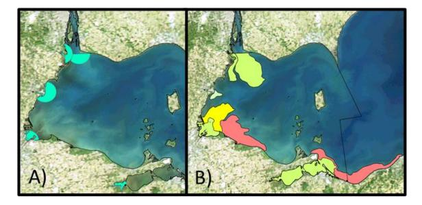
Figure 15: River plume layer development A) initial concept based on a 5km buffers around river mouths, transitioned into B) plumes delineation based on orthoimagery that define plume area and relative intensity gradient with highest plume intensity (green), moderate intensity (yellow), and minimal intensity (red).
