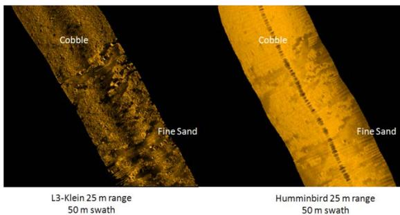
**Figure 2. Comparison of sidescan sonar images. North of Painesville Township Park. Water depth: 25ft L-3 Klein: 500 kHz (left) Humminbird :455 kHz (right)**
