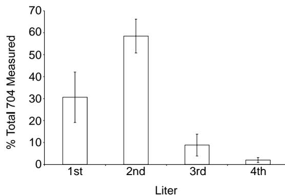
Fig 10. Quantities of 704 that were measured in each successive liter of methanol as XAD7HP resin was eluted. N=3 extractions. Bars are average % total 704 measured, error bars are one standard deviation. Results for PS and 590 were similar.
