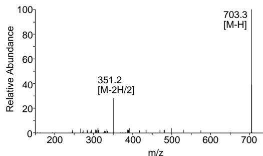
Fig. 1. Mass spectrometry of 704 using electrospray ionization with an ion trap in the negative ion mode. The  $[M-H]^-$  ion can be seen at 703.3 m/z; the dianion at 351.2 m/z. UNPUBLISHED DATA, PLEASE DO NOT CITE OR DISTRIBUTE
