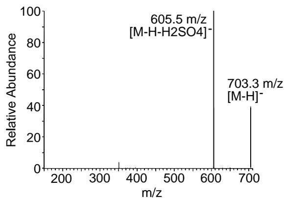
Fig. 2. Mass spectrometry/mass spectrometry of 704 using electrospray ionization with an ion trap in the negative ion mode at 30% collision energy. The  $[M-H]^-$  ion is seen at 703.3 m/z; the fragment peak representing the loss of  $H_2SO_4$  at 605.5 m/z. UNPUBLISHED DATA, PLEASE DO NOT CITE OR DISTRIBUTE
