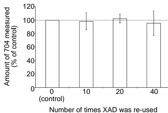
*Fig. 11. A measure of the ability of XAD7HP to repeatedly extract 704 from larval holding water. Larval water was passed through XAD7HP either 10, 20 or 40 times, and the resultant 'used' XAD was then compared to new 'unused' XAD. The amount of 704 was quantified in each extract using ESI-MS and expressed as a percentage of 704 in the control. Bars are an average of 3 separate extractions, error bars are one standard deviation. Results for 590 were similar.*
